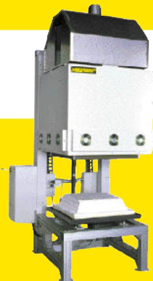
In addition to the furnaces presented here, we also deliver compact bench-type models, chamber furnaces with state-of-the-art lift-top technology with up to 2000 litres useful volume as well as individual solutions based on customer requests.
