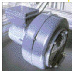
As an option: Supply air blower for cooling or with air preheater for debinding...
