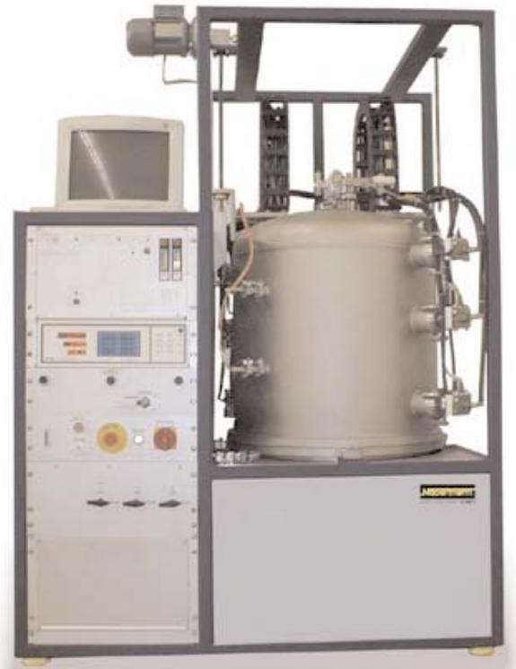
Top-hat furnace for protective gas and vacuum annealing of small parts
