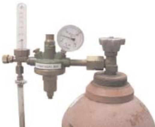
Manual purging equipment with pressure reducer and flow meter
