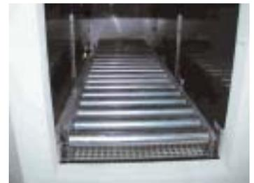
Example: Roller conveyor in the convection furnace for annealing of rod and strip
