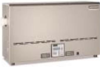
Tube furnace for normal atmosphere
