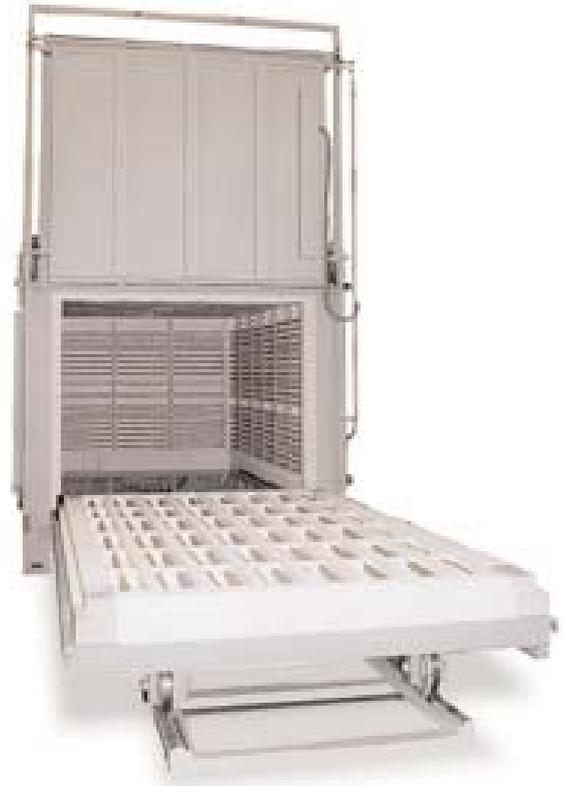
13 m<sup>3</sup> bogie hearth furnace for annealing large parts of up to 12 tonnes
