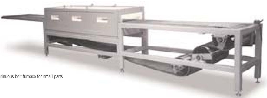
Continuous belt furnace for small parts
