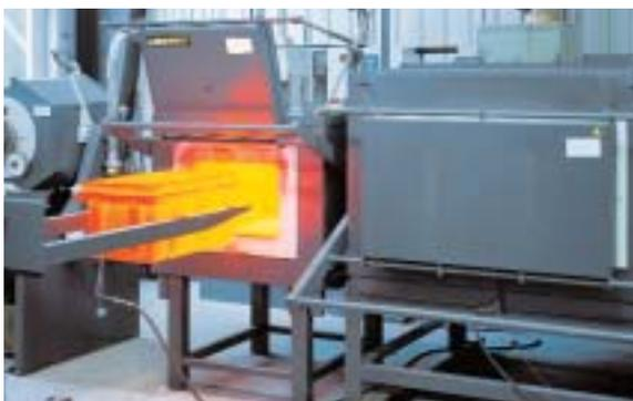
Powder boronising in a chamber furnace
