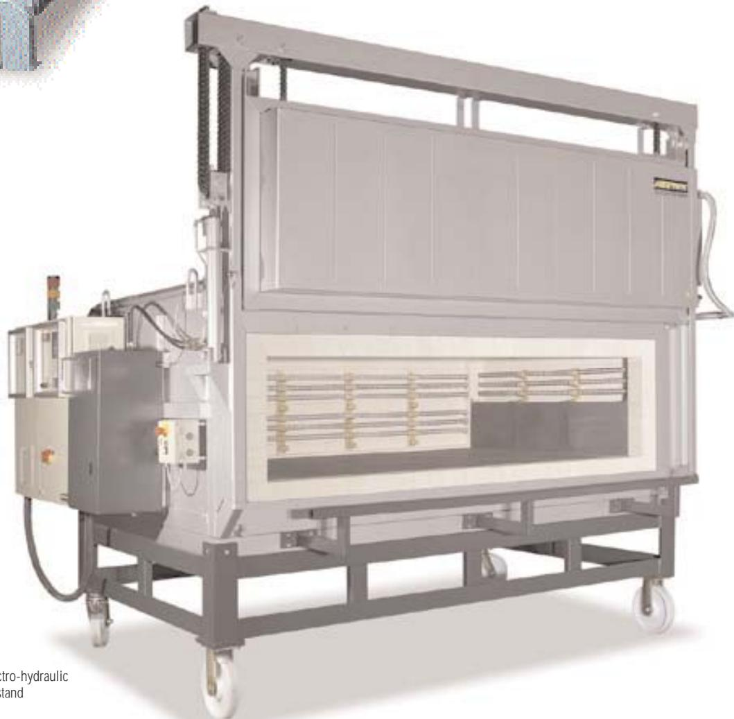
Annealing furnace with electro-hydraulic lifting door and moveable stand
