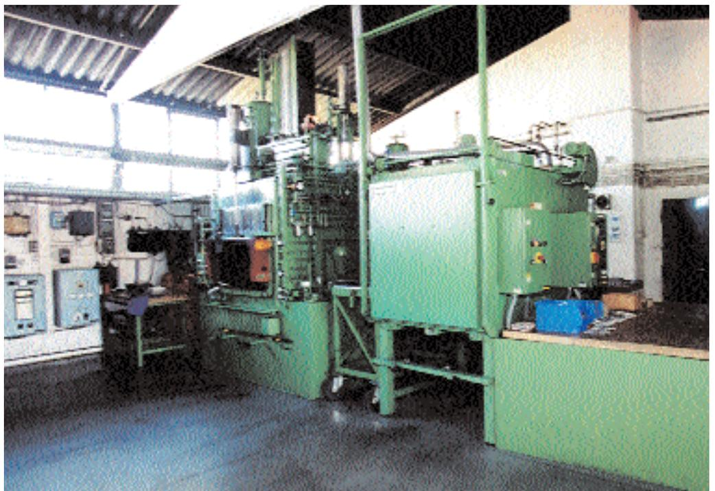
Protective gas convection furnace for bright tempering and bright annealing in contract heat treatment
