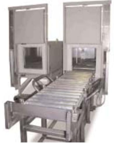
Example: Convection furnace with cooling station and roller conveyor
