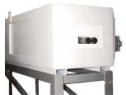
Furnace with two tubes for annealing of strip
