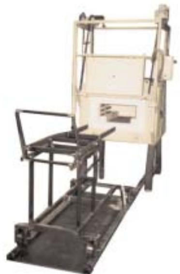
Semi-automatic chamber furnace with guided charging device
