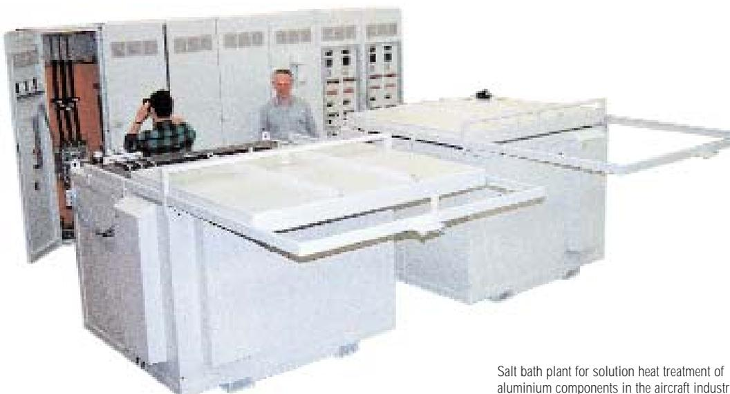
Salt bath plant for solution heat treatment of aluminium components in the aircraft industry
