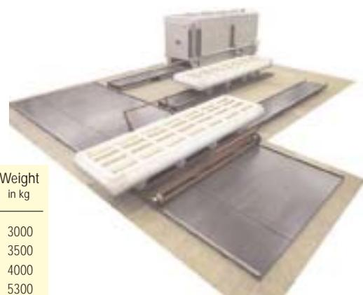
System with several furnaces with cross transfer car and centralised control
