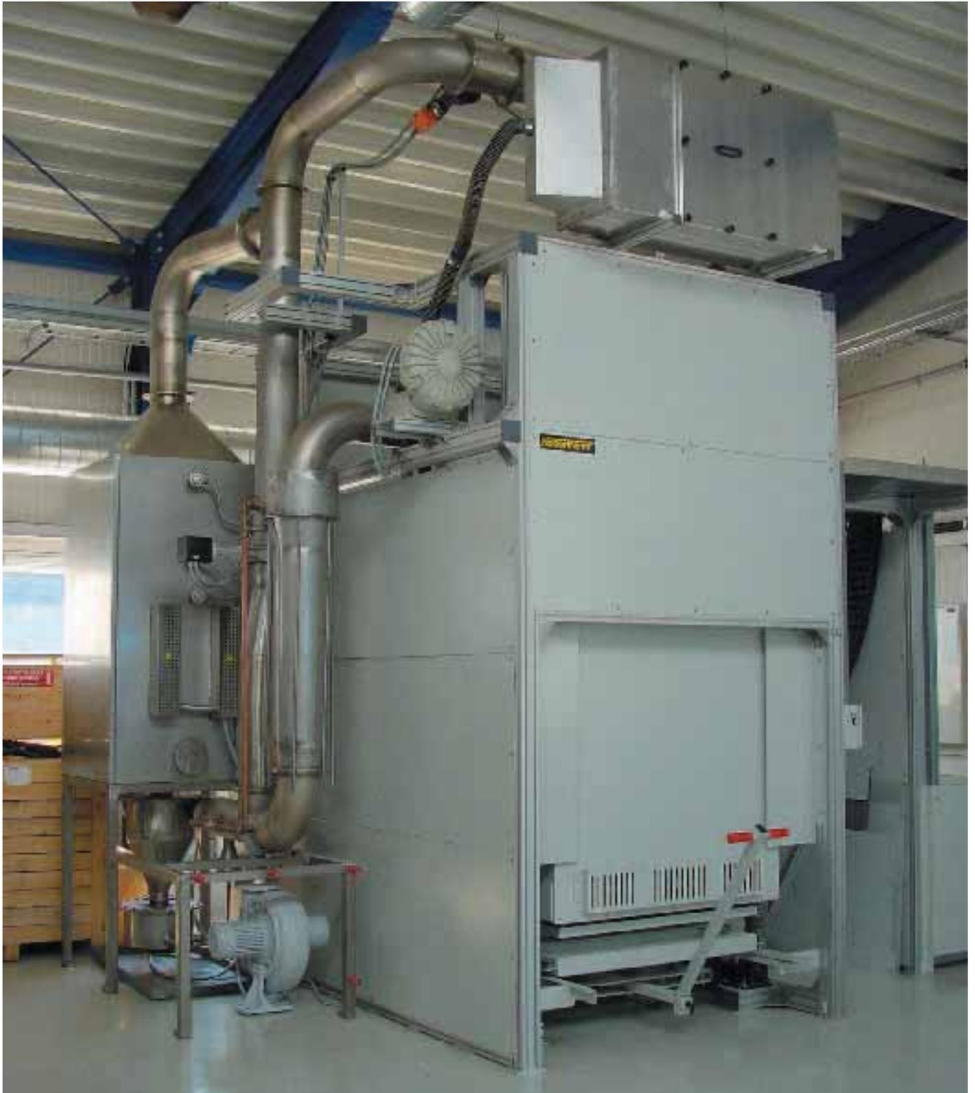
High-temperature combi-plant unit **HT 1440/17 LTS** for debinding and sintering
