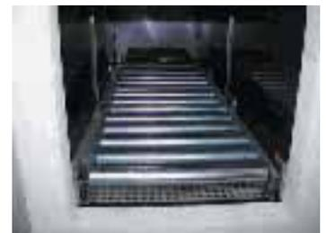
Roller conveyor in the furnace
