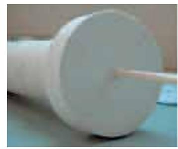
Fibre plug with protective gas connection
