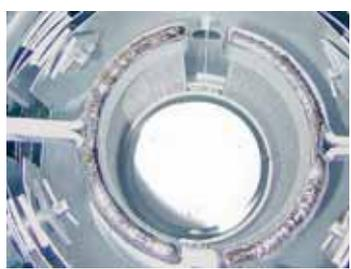
Molybdenum/Tungsten heating chamber
