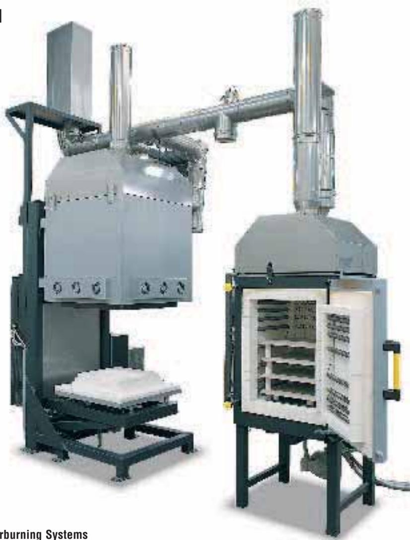
Debinding and sintering plant with catalytic afterburning system
