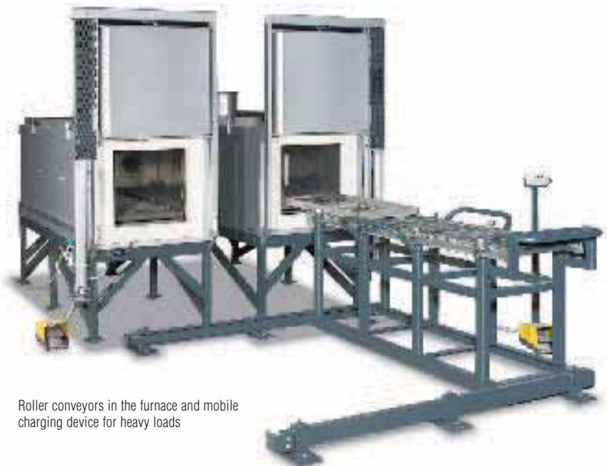
Roller conveyors in the furnace and mobile charging device for heavy loads
