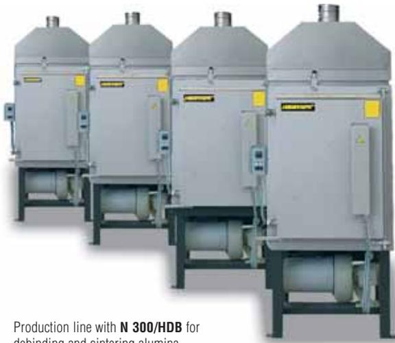
Production line with **N 300/HDB** for debinding and sintering alumina
