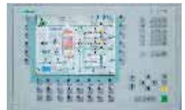
PLC fully automatic furnace control
