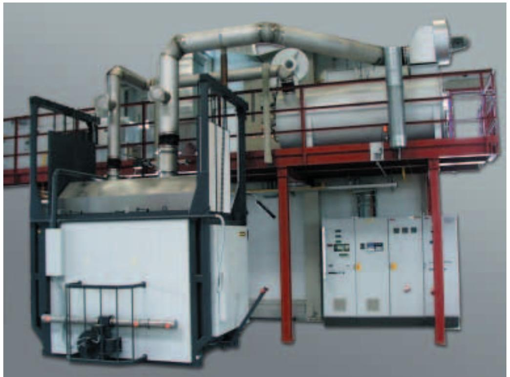
**W 2640/GS with thermal afterburning system**
