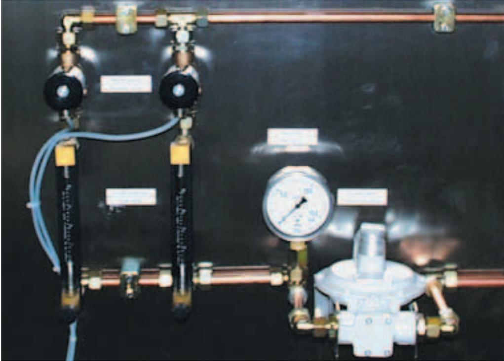
For work done under controlled atmospheres we supply gas purging systems. These are basically available for all types and models, customized to suit the respective process conditions.
