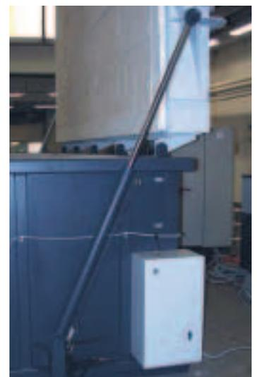
Electro-hydraulic powered furnace lid
