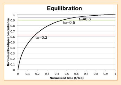
The C-sense will reach the t63 level in  $\sim 3$  minutes. The total time is about 15 minutes but this can be reduced to about 12 minutes if you use a water-pumped head. The analog output updates at once per second.
