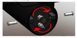
4) Insert the retaining pins through the predrilled holes in the C-ray's housing and through the eyelifts on the C3's housing thereby retaining the C3's position.
