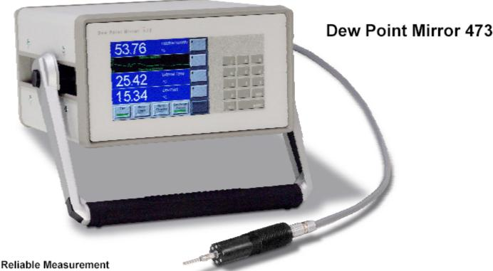
The Model 473 Dew Point Mirror is a portable instrument equipped with a separate measuring head for both spot and continuous measurement of Dew/Frost point and temperature in air and gas mixtures. Based on the chilled mirror principle, the 473 ensures direct and accurate humidity measurement.
