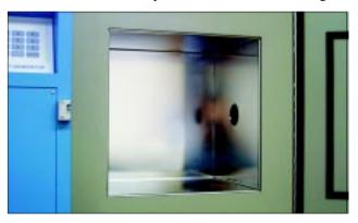
Virtually any humidity and temperature point may be generated, for any length of time, within the operational limits of the generator. The output of the device under test may then be compared with the generator's printed data for analysis.
