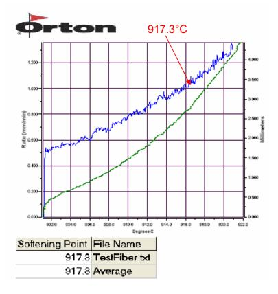
Operating Modes: The Orton SP Software prompts the operator to select one of two modes of operation: the ASTM C-338 Mode, or the User Defined Mode. The User Defined Mode follows the guidelines of the ASTM C-338 Mode, but allows the operator to change the test parameters (the starting temperature for each test, the heating rate for the data collection period, and the target elongation rate) to suit individual testing requirements.
