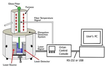
The software directs the PID controller to follow the thermal cycle, collects the data signals from the sample thermocouple and laser, displays the data on the computer monitor in real time, performs the appropriate calculations on the data, stores the data and calculations in a text file on the hard drive, and waits for the operator to begin the next test. The software also opens past data files for post testing review, analysis, and report generation.
