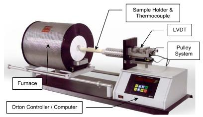
certification. Orton standard dilatometers are used for ASTM E-228, ASTM C-372, ISO 7991, and other testing procedures to measure the Coefficient of Thermal Expansion (CTE), softening point, glass transition temperature, curie point, crystalline transformation, phase transition, shrinkage, warping, bloating, sintering rate, isothermal creep, stress relaxation.
