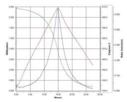
**Data Acquisition:** The graph at the left is the real time display of the test procedure. The computer continuously monitors and displays the LVDT and thermocouple outputs, and calculates and displays the rate of deflection:
