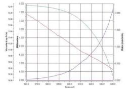
Data Analysis - ASTM C-1350M: At the end of the test, the computer software plots the deflection and deflection rate versus temperature, and calculates the viscosities at various temperatures according to the equations in C-1350M. This analysis is performed automatically WITHOUT the operator, so OPERATOR ERRORS and BIAS in data analysis are **ELIMINATED !!**
