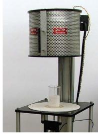
manually raised and lowered furnace for easy sample loading and unloading, a 2point sample support system, a midpoint sample load rod hook, a set of weights, an LVDT system to monitor continuously the sample deflection, the Orton BBV Controller Console, Orton BBV Software, and a dedicated personal computer system.
