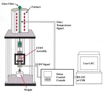
on the computer monitor in real time, performs the appropriate calculations on the data, stores the data and calculations in a text file on the hard drive, and waits for the operator to begin the next test. The software also opens past data files for post testing review, analysis, and report generation.
