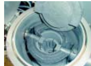
Graphite heating chamber
