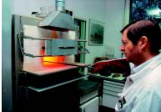
N 110/HS1 with lifting door for gold melting trials
