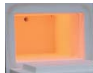
ceramic retort with heating on all sides
