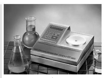
concentration of CIP solutions. The LR-01 has internal alarms that can be set to detect variations from target values, and can be connected to a computer and standard printer.
