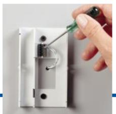
Wiring is connected to the terminal block in the base and the cover can be snapped into place at a later time. This feature is especially attractive when a transmitter will be incorporated into new construction because it lets the user mount and wire the unit without the sensor and electronics, thereby avoiding possible damage from rough handling or contamination from paint and dust.
