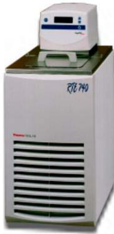
Figure 8. Temperature controlled bath/circulator used to circulate water through the water bath of the Humilab.
