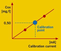
Linear correlation between oxygen concentration and calibration current
