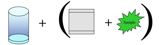
Insert filter bag/sample into crucible and ash
